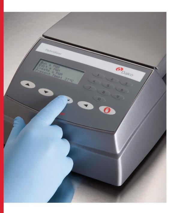
Hybridizer is a hands-free, codenaturation and hybridization instrument designed for slidebased fluorescence (FISH) and chromogenic (CISH) in situ hybridization on histology and cytology samples.
